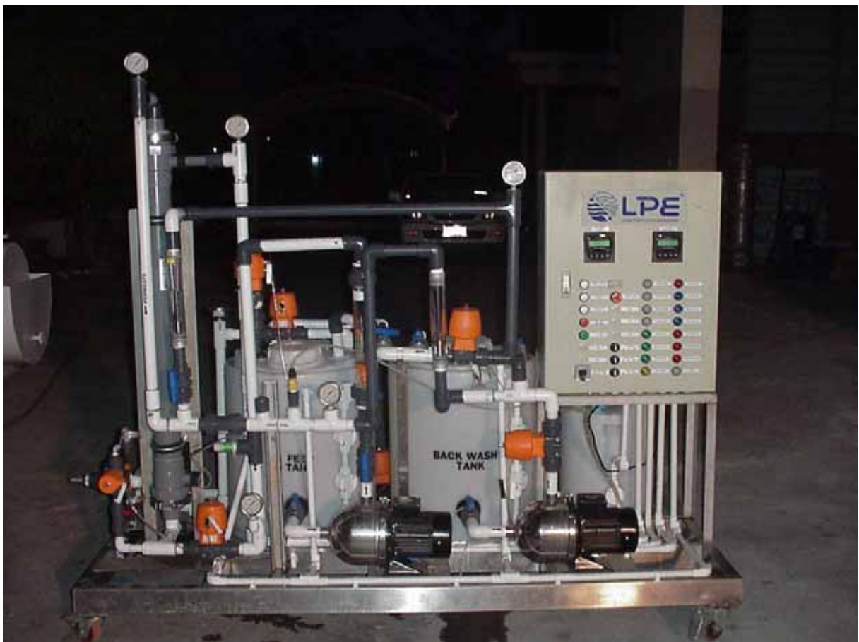
Figure 3.9 The Microfiltration Membrane Pilot Unit
