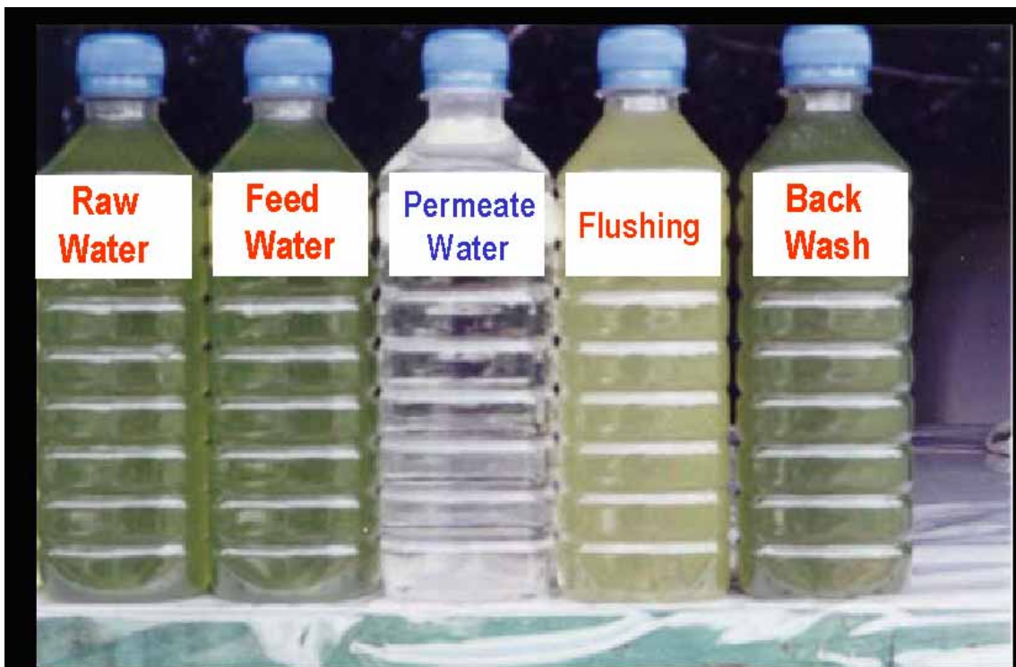
Figure 4.27 Water Quality in Case of Secondary Treated Wastewater as the Raw Water
