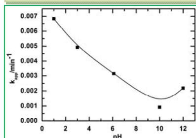
Fig 4: pH effect on apparent first order kinetic constant ( $k_{app}$ )
