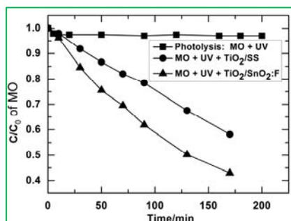
Fig2: Kinetics of the disappearance of Methyl Orange (MO, 1 mM)
