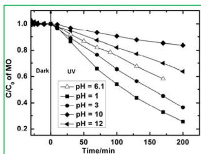
Fig3: Effect of the pH on MO degradation
