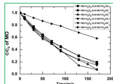
Fig5: Effect of H<sub>2</sub>O<sub>2</sub> and S<sub>2</sub>O<sub>8</sub><sup>2-</sup> on MO degradation
